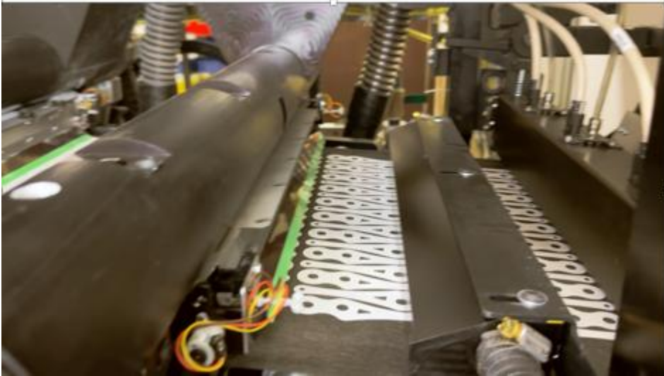
The vision system checks printed images to match the intended design
