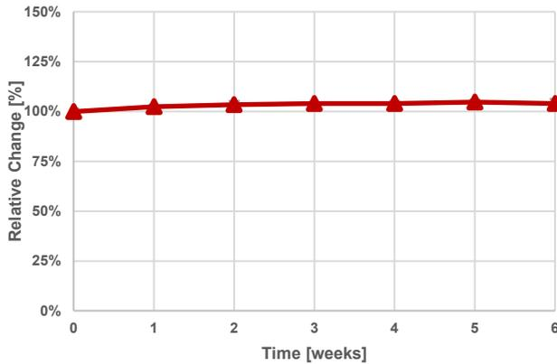
Flexural Elongation at Break after Heat Ageing at 50°C
