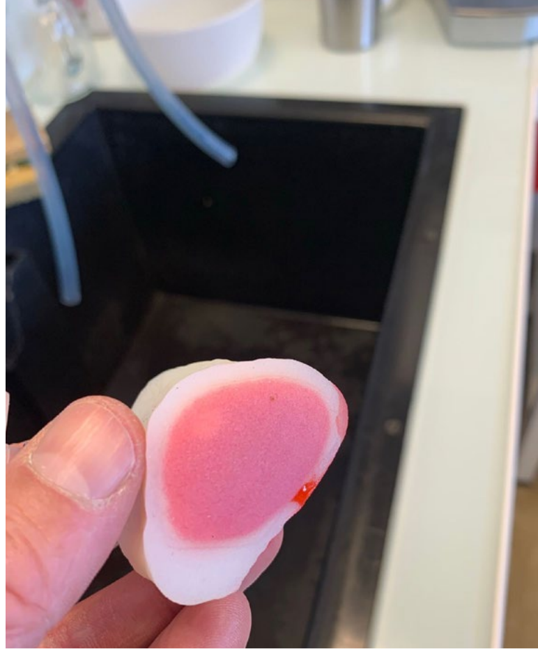
The J5 MediJet’s multi-material multi-color 3D printing capability enables the production of ultra-realistic models for pre-surgery preparation and training
