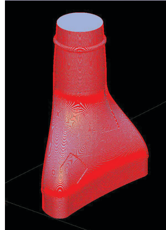
Figure 1 - FDM sacrificial tooling is easily created from the CAD model of the composite part and prepared for building using Stratasys Insight software.
